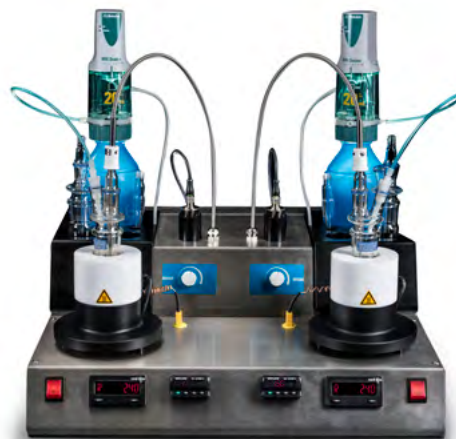
Automated Stability Analyser Method: ASTM D7060-12
